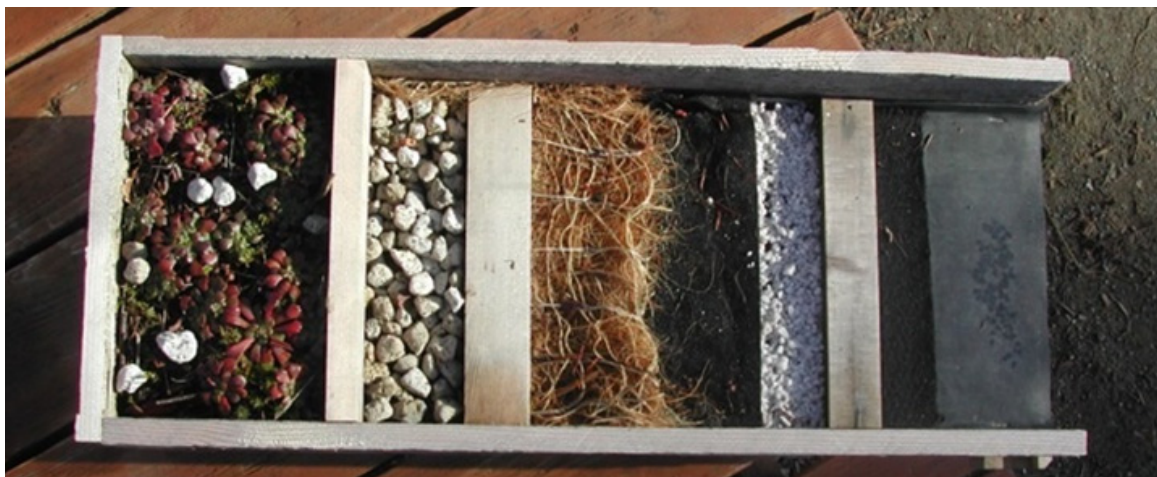
Figure 34: Model of Living Roof Layers
