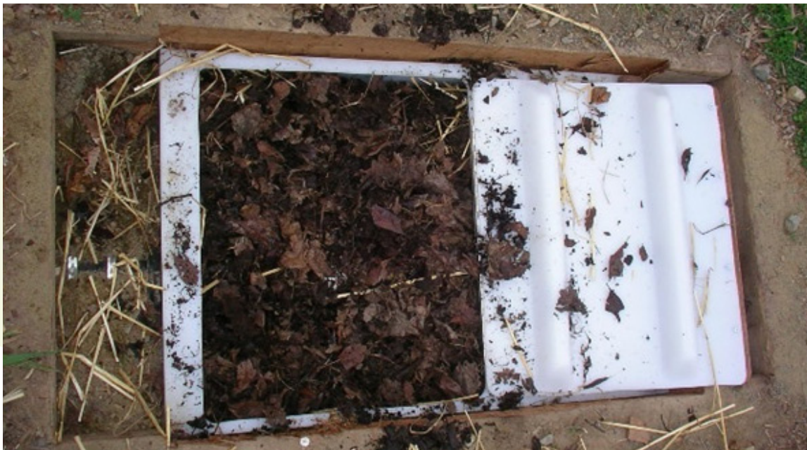
Figure 37: Worm filter system
